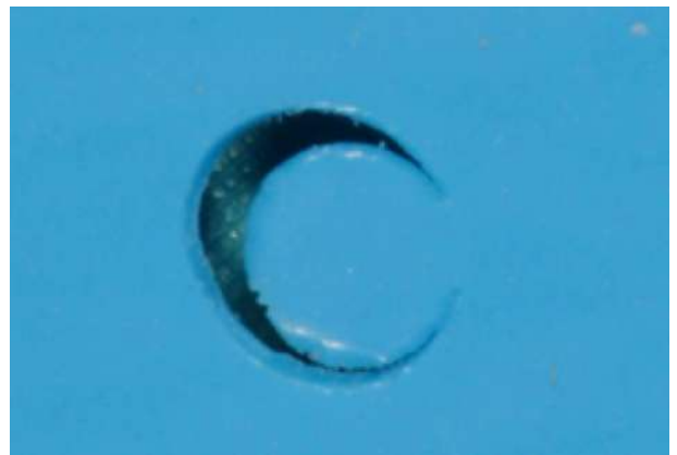
Fig. 13. If the hole-punching revolving head is worn down, the piercing will be incomplete.
