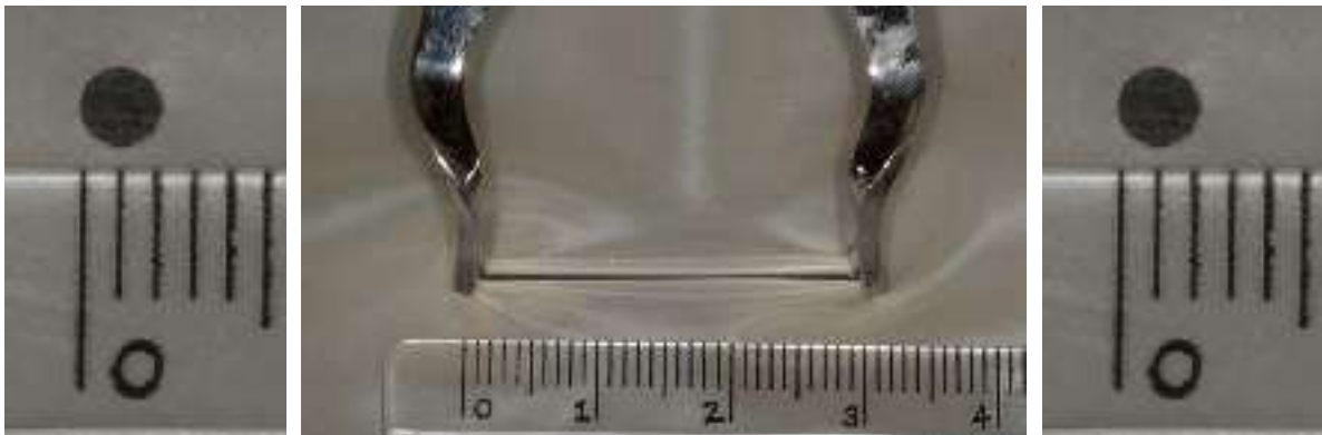
Fig. 1-3. Amongst punch plier holes, the biggest one has a diameter of about 2.3 mm. Due to latex elasticity the hole can be stretched open up to 3 cm without tearing. Once the pressure is removed, the hole takes back its original shape due to latex resilience .
